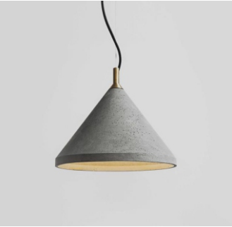
Pendant Lamp · ren Material: Concrete, Aluminum Alloy / Brass Size: Ø300×h260 mm Weight: 1.9 kg Cord: Black, 2 m Bulb Type : E27 LED Wattage / Voltage: 9W / 85-265 V
